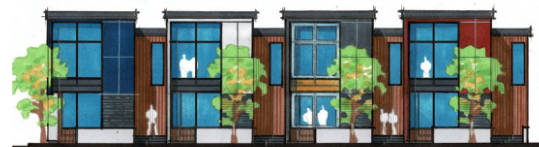
WALL SYSTEM #6 BRICK MASONRY BY 'MUTUAL MATERIALS' OR APPR. COLOR: 'BLACK'
