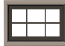
WINDOW/DOOR #1 METAL CLAD FRAMES ANDERSON '100' SERIES, 'WESTERN', OR APPR. COLOR: BLACK
